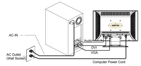
Note: Turn off your PC and the LCD monitor before connecting your LCD monitor to the computer.
